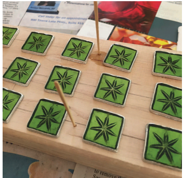
Fig 15 - Toothpicks to keep foil away from mounts
