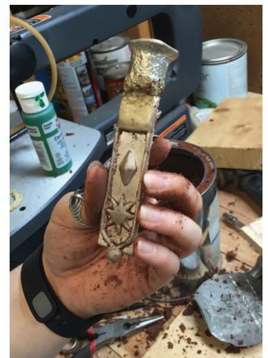
Fig 12 - Cast belt tip removed from sand
