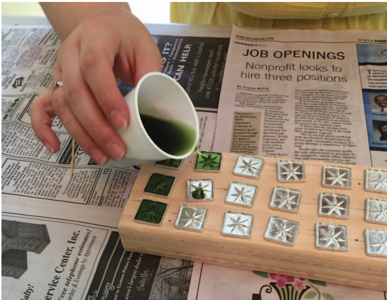
Fig 14 - Pouring resin into belt mounts
