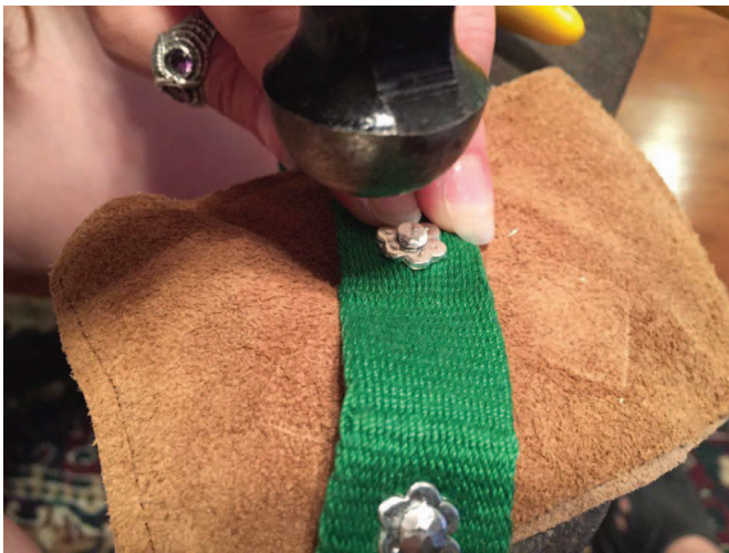
Fig 18 and 19 - Clipping rivet and peening rivet
